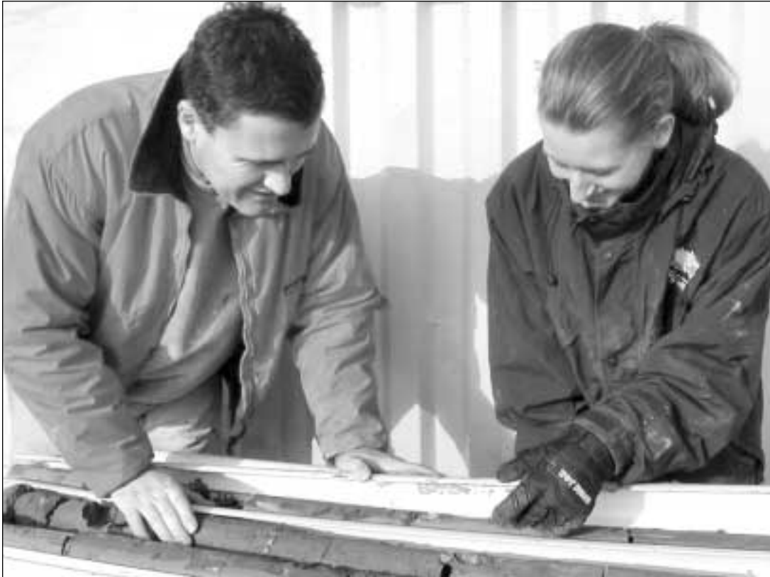
Geologist Steve Davies and assistant Kim Gilder look over some core samples taken from a new Oak Ridges Moraine monitoring well being constructed in the Centreton area. When drilling is complete, geologists will have samples of all soils found from ground level to bedrock, giving a snapshot of the moraine's formation.
